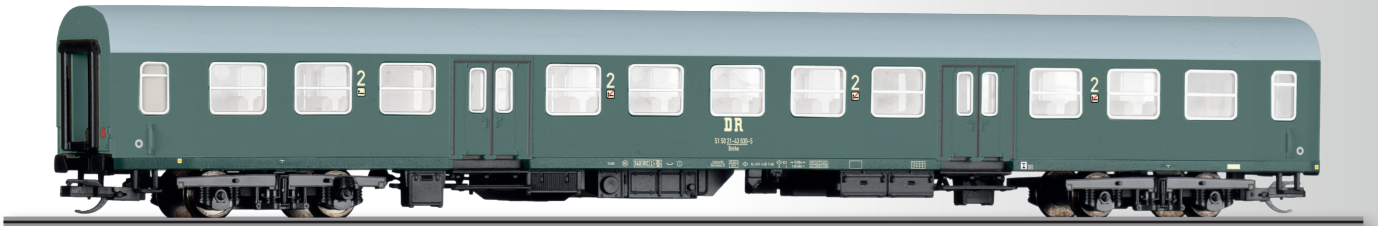
Reisezugwagen 2. Klasse Bmhe der DR 2nd class passenger coach Bmhe of the DR
